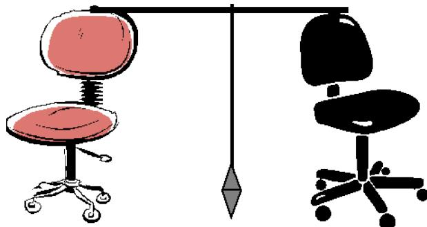
5. Start the weight swinging and time how long it takes to make 20 swings. Use a stopwatch for this.
